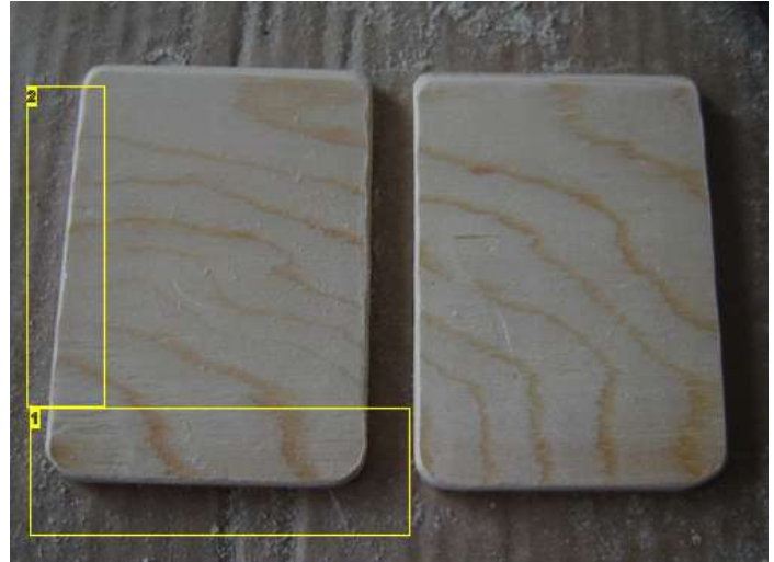
Image Notes 1. Round the corners so that it is more comfortable to place in your pocket. 2. Smooth the edges of the wood.
